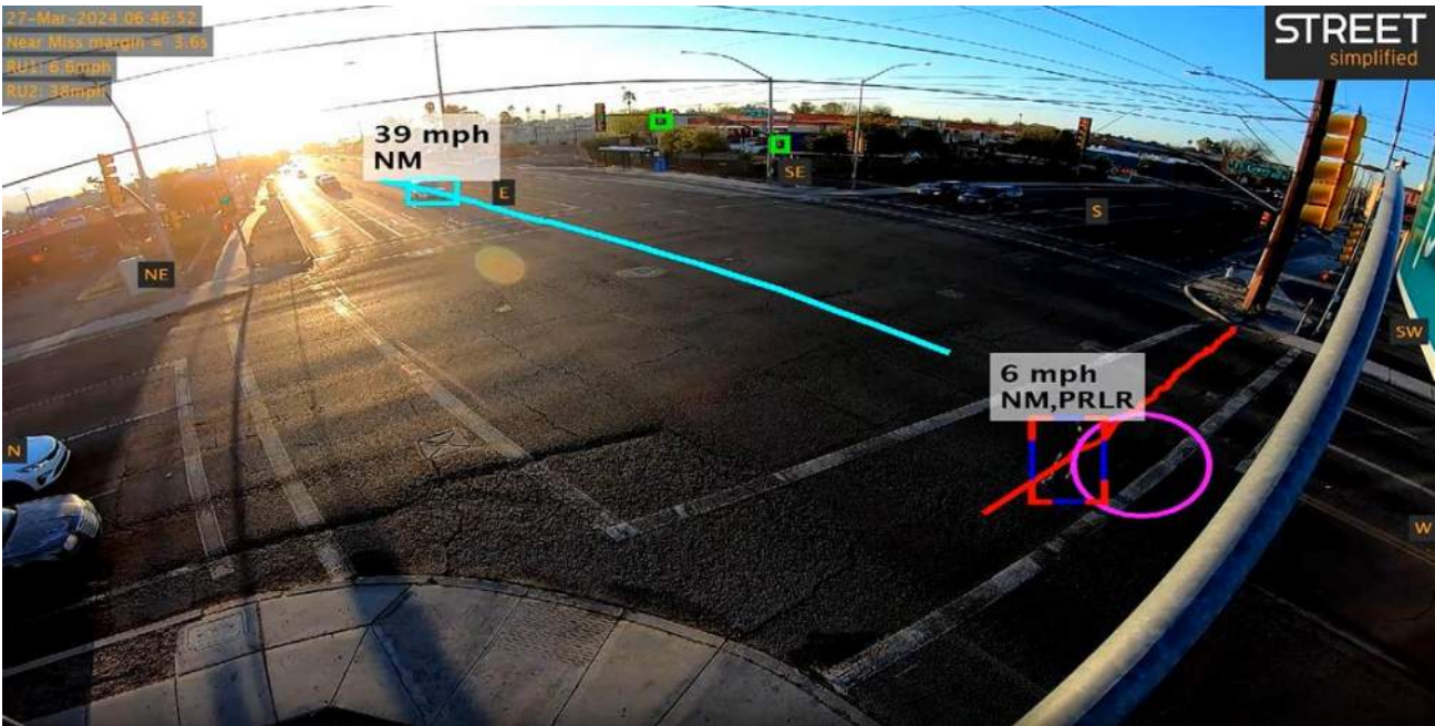
Figure 41. Fort Lowell intersection near-miss involving a pedestrian crossing during the don't walk phase
